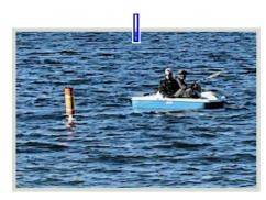
ICESPY is installed like a buoy. Simply put it in the water, drop the anchor, and turn on the power switch.
