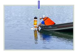
LAKESCOUT is installed like a buoy. Place the anchor at the bottom of the lake and turn on the power switch. LAKESCOUT can also be deployed in the winter by cutting a hole in the ice and dropping it in place.
