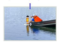
PONDWATCH is installed like a buoy. Place the anchor at the bottom of the pond and turn on the power switch. PONDWATCH can also be deployed in the winter by cutting a hole in the ice and dropping it in place.
